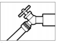
Step 4 Connect garden hose to the cold water source and turn water on completely.
